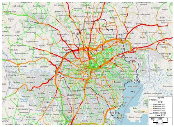
Figure 13.4.8 AM Peak Private Vehicle Volume to Capacity Ratio and Flow Volume in KCC, 2021 Base Scenario
