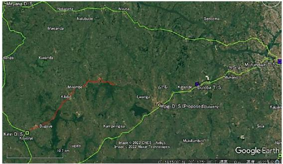
Note: Green line: Existing 33kV incomers. Red line: existing 11kV feeder Source: JICA Expert Team
